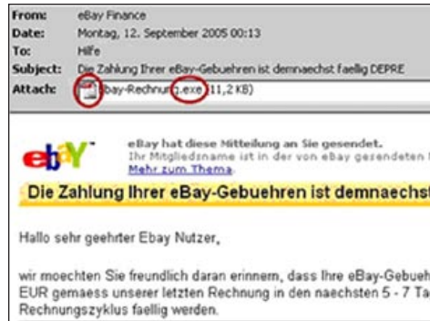
Localized mail with an invoice Trojan carrying a fake Adobe Acrobat Reader icon.
